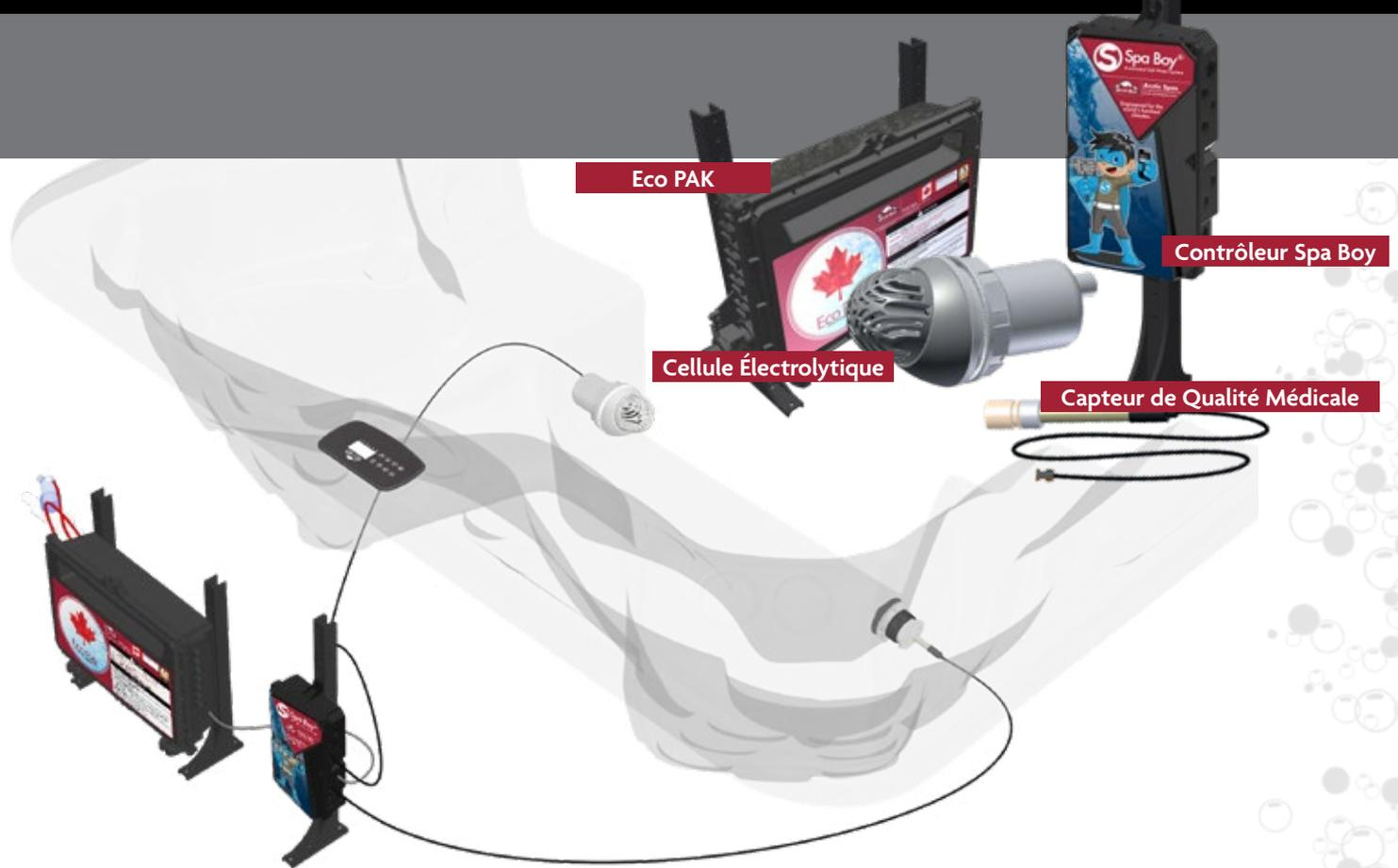
A **medical grade sensor** measures ORP and pH for water quality. The **Spa Boy® controller** analyzes the data and activates the **electrolytic cell** when the water quality drops below the set point. The **EcoPack** control system integrates Spa Boy® with the main hot tub controls and enables 2 way communication with the Arctic Spas App or [myarcticspa.com](http://myarcticspa.com) via the internet.
